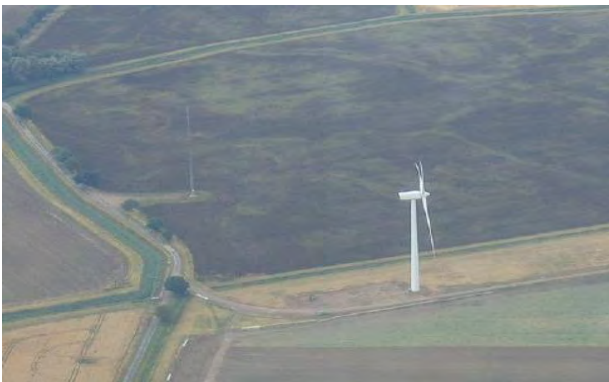
Figure 3: Difficulties in visually acquiring anemometer masts.
