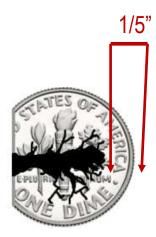
In the event of a stress crack, the allowable width of the remaining cask wall is a dangerously narrow 79/500<sup>th</sup> of an inch, or less than 1/5"
