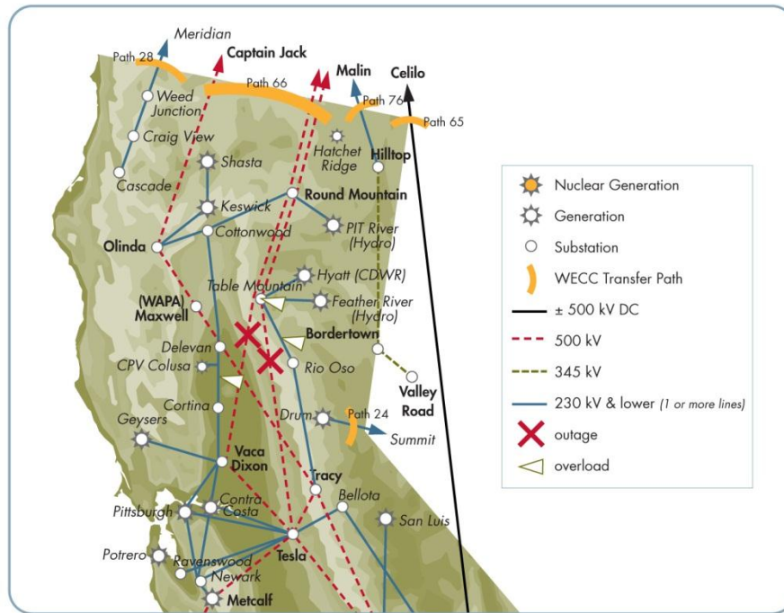
Figure 2.4.4.1-1 PG&amp;E Bulk Transmission System Overload in the Table Mountain area
